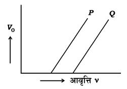
The graph between the stopping potential  $V_0$  and frequency v for two different metal plates P and Q are shown in the figure. Which of the metals has greater threshold wavelength and work function?
